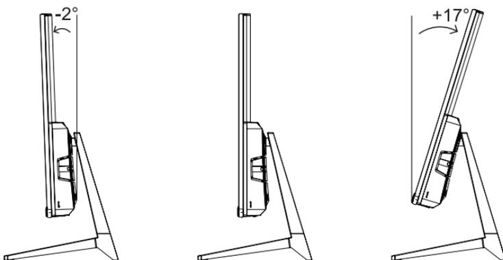
Stand the monitor up and adjust the tilt angle of the monitor as needed
