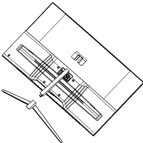
Take out the bracket, align it with the interface on the back of the display, insert four screws and tighten it with a screwdriver; Insert the base interface into the bracket, insert a screw, and tighten it; finally put the decorative plastic cover in and fasten.
